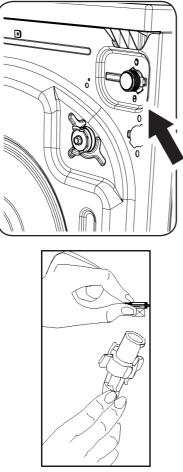
• Remove the filter of the water inlet valve on your machine with a pair of pliers. Clean thoroughly using water and a brush.
