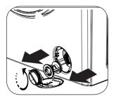
• Loosen the filter cover by turning it counter-clockwise, and remove by pulling.
