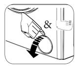
• You may use the washing powder spade supplied with your machine or liquid detergent level plate to open the pump cover.
