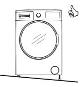
You can adjust the balance of your machine by a gauge from the top.
