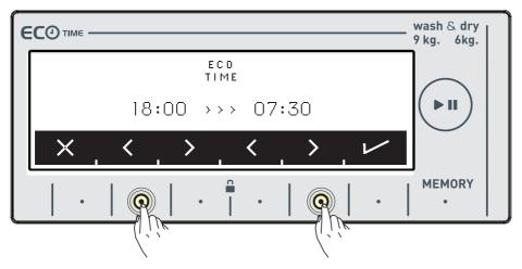
• You can adjust the Eco Time interval by touching the buttons of symbols  $\langle \rangle$ See page 60 to activate the Eco Time interval additional function.
