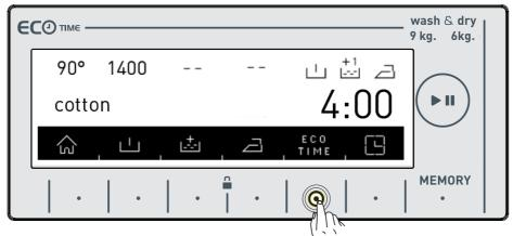
• If you want to run a program while the eco time feature is active, touch the button of • symbol. The starting time of the programme will automatically be delayed until the economic time interval. The programme "starting time" and the programme duration will be shown on the display with certain intervals.
